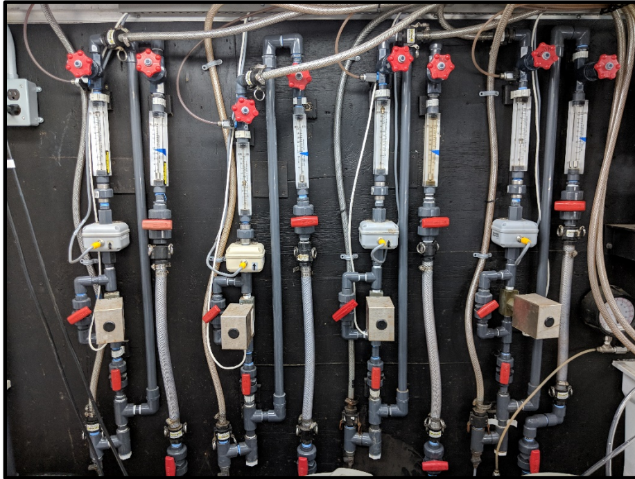
Figure 2.07: Flow Control for Pilot Filters
